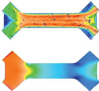
RefleX Chamber design creates a highly turbulent flow for uniform treatment without shadowing or dead spots.
