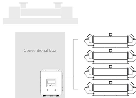
Typical control boxes only operate one chamber at a time. Compact RefleX controllers can run up to four chambers independently in a smaller footprint.
