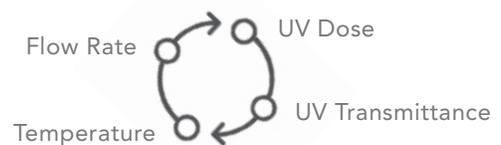
Determining the optimum level of UV disinfection for a given application involves a mix of four critical performance variables: flow rate, required UV dose, percentage of UV transmission and operating temperature.
