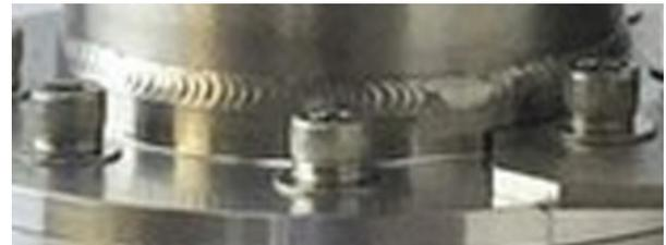
Look for stainless steel with plasma-fused welds for contaminant-free components.
